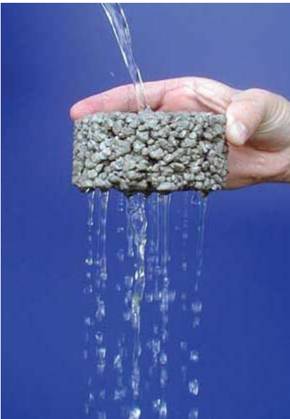
A sample of pervious concrete that shows its effectiveness in shedding rainwater.
