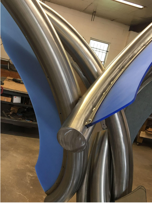
Images: acrylic mounted in a channel welded to the large stainless steel curve and attached with isolation material and fasteners.
